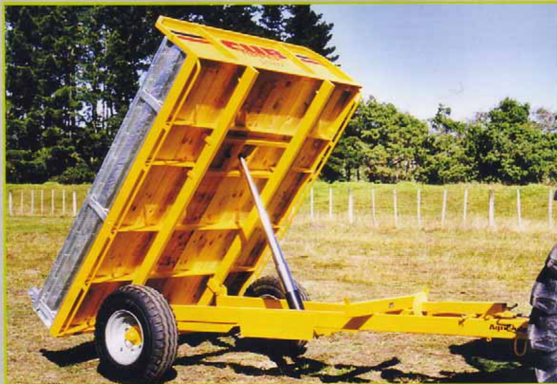
3 Ton Tipper in unloading position 53° angle
