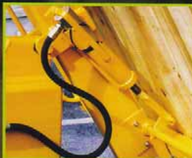
hydraulic auto-release tailgate
